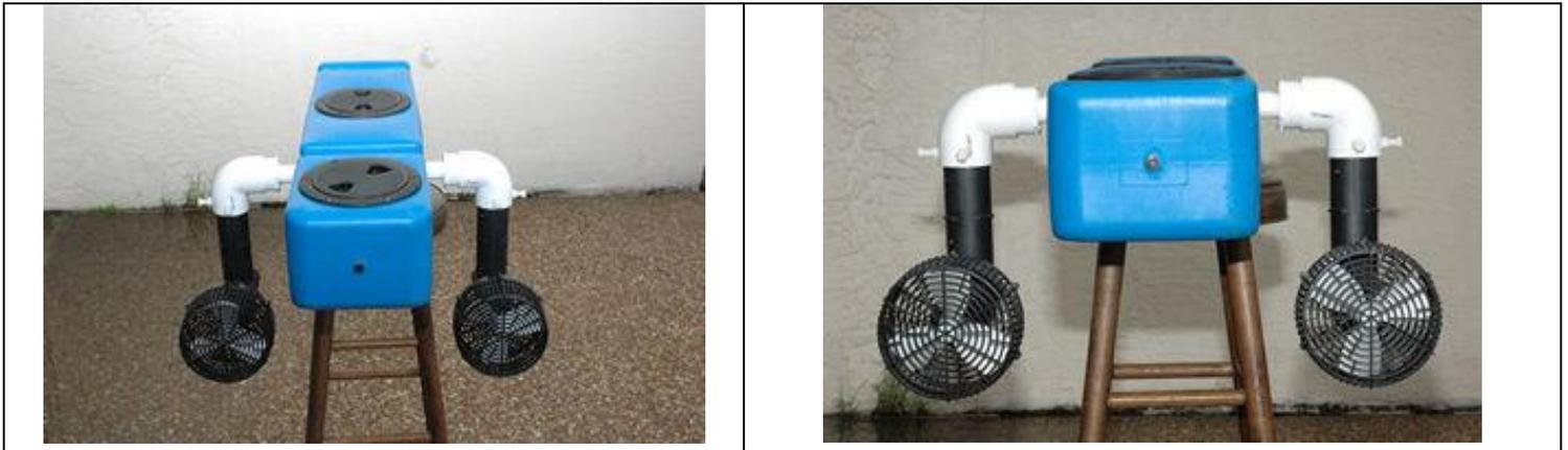
The next step was to build the “sensor pack”, this is the PVC framework where the “whisker switches” and infrared detector will be mounted. Once again, the original molded-in nuts in the hull were utilized
